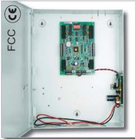
IRC-2000 Includes controller, ENCL1 enclosure and PS1224 power supply.
